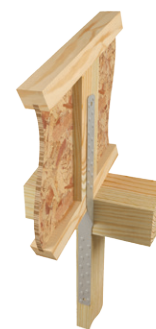
Typical MTW20 I-joist Rafter installation
