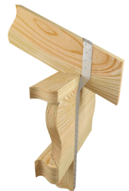
Typical MTW30 I-joist Rafter installation
